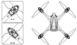
Attach the propellers to the corresponding motors that are marked with A and B,tighten the propellers and keep the motors deadlocked with the screw-driver.
