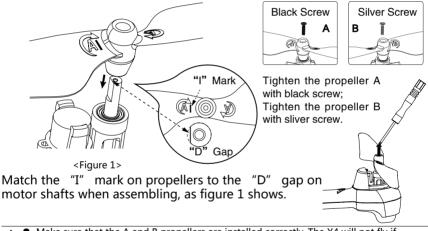
Make sure that the A and B propellers are installed correctly. The X4 will not fly if propellers are improperly installed.
